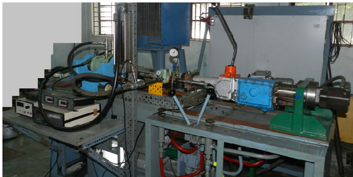
Test rig for LSHT Hydrostatic Unit Performance Test Rig.
